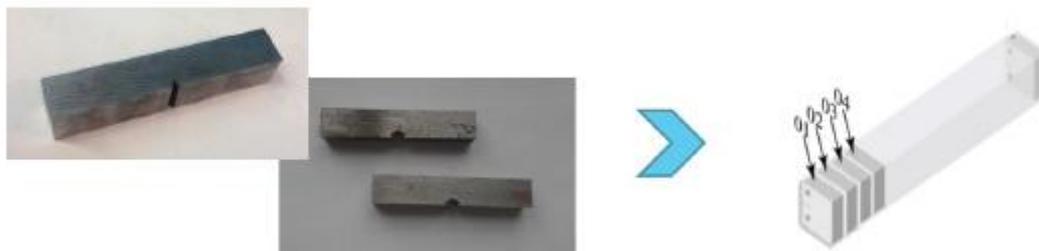
Figure 44: Illustration of the CT0,16T specimens which can be made from broken pieces of Charpy and COD specimens
