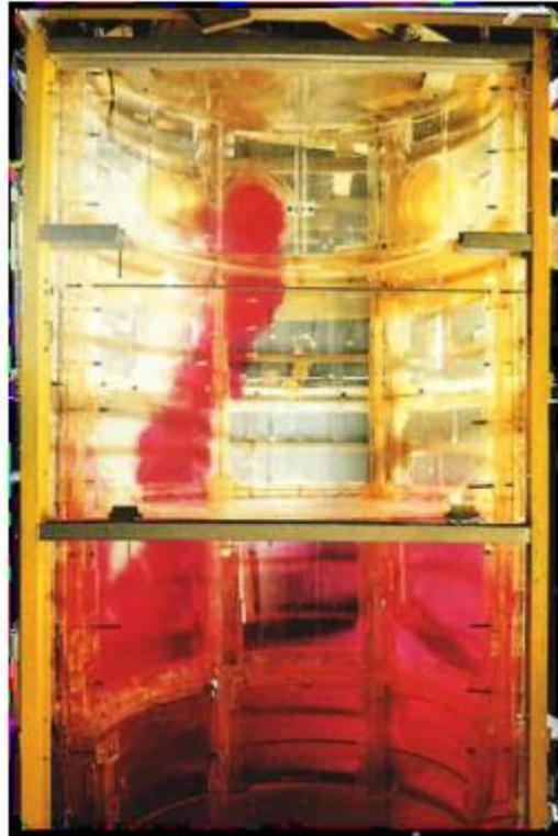
Figure 42: Thermal mixing experiments for Loviisa reactor pressure vessel in scale 2:5.
