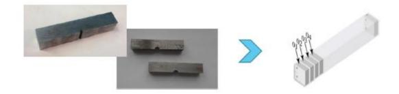
Figure 44: Illustration of the CT0,16T specimens which can be made from broken pieces of Charpy and COD specimens
